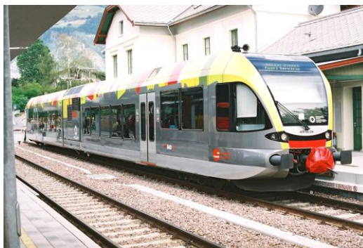
DMU (Stadler) with Syope wheels on the Val Venosta line (photo: Pippert)
