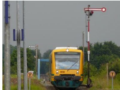
Regio Shuttle (Stadler) : DMUs of the same basic design but upgraded for Stage IIIb will be used on the VBB network
