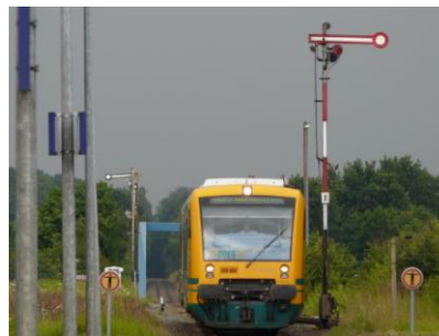
Regio Shuttle (Stadler) : DMUs of the same basic design but upgraded for Stage IIIb will be used on the VBB network
